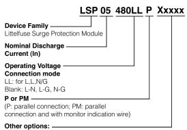
X3333: with GND wire connection, available for 240Vac and 277Vac rating with CE Marking for Class I earth installation.
